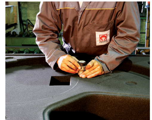
Strength check on cured mould and core
